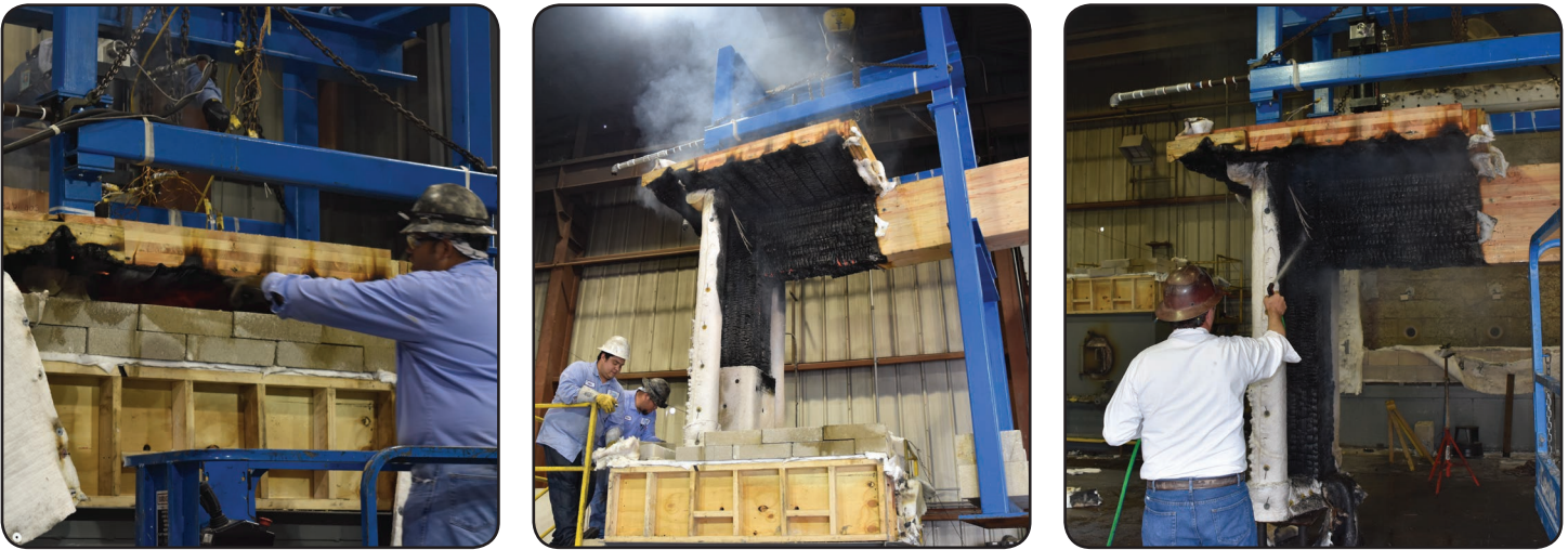
Figure 5. Opening of furnace (left); removal of specimen (middle); extinguishing of specimen (right).
