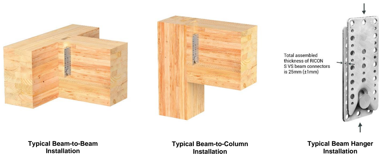
FIGURE 2—RICON S VS SERIES BEAM HANGER INSTALLATION
