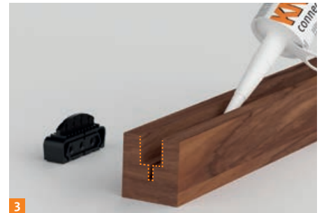
3 Mill a 2-level groove and fill it with KNAPP® PU+ adhesive or apply the adhesive on the block rail. Clip the workpiece onto the clamp.
