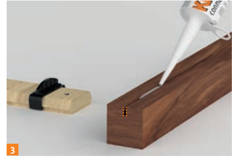
3 Mill a 4x12 mm groove and fill it with KNAPP® PU+ adhesive or apply the adhesive on the block rail. Fix the decorative moulding onto the block rail.
