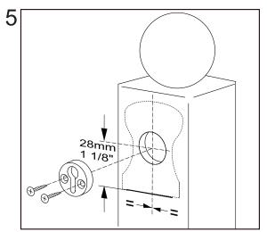
To mark the centre of the keyhole disc measure 1 ½" (28mm) upwards from the bottom of the rail position. Using a 1" (25mm) bit bore hole into post ½2" (7mm) deep so the keyhole disc is flush or slightly under. Secure disc with screws, bore pilot holes first.
