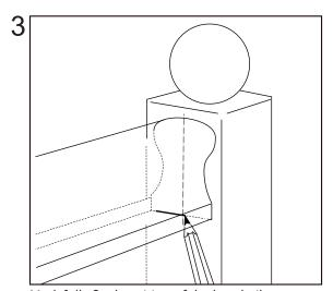
Mark fully final position of the handrail onto post observing the centre line.
