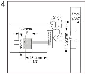
Insert connector into rail, check travel left to right.
