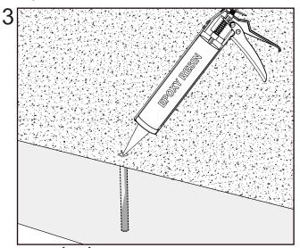
Fill hole ½ to ½ with epoxy resin.
