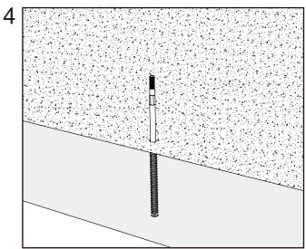
Set shaft at correct height and wipe off excess epoxy. Allow to set.
