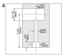
**4.** Mark the center point of the 1 1/2"-38mm hole on side of the post and bore to recommended depth. Mark the center of the post base and bore the 1"-25mm hole 3/4"-19mm deep. Now using a 5/8"-16mm continue boring through the centre of the 1"-25mm hole until reaching the 1 1/2"-38mm hole. Ream the 5/8"-16mm hole if necessary. The 1"- 25mm hole allows the post to sit freely over the hex nut on the Base Plate.
