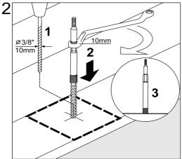
**2.** Bore the center pilot hole 3/8"-10mm. Tighten lag end into the wood with 10mm wrench stopping at the point of the machine thread that will receive the Base Plate. If needed, use some wax for lubrication on the lag portion of shaft to ease installation.
