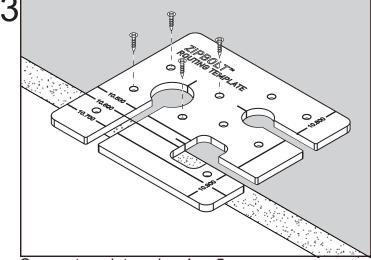
Secure template using 4 or 5 screws.
