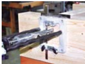
Manual drilling using a stepped drill bit or industrial drilling on a CNC machine
