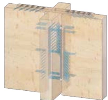
MEGANT® main secondary beam connection with T-JOINT D35 W30 screwed-on hardwood tension ties.
