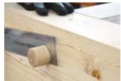
Cut and sand the excess part
